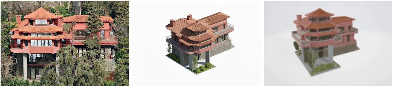
Figure 4. Three-step workflow of the proposed method illustrated using the Bruno Taut Villa: (left) original building photograph, (centre) isometric daylight image generated by Gemini Flash 2.5, (right) textured 3D building model reconstructed by Hunyuan3D 2.1.
