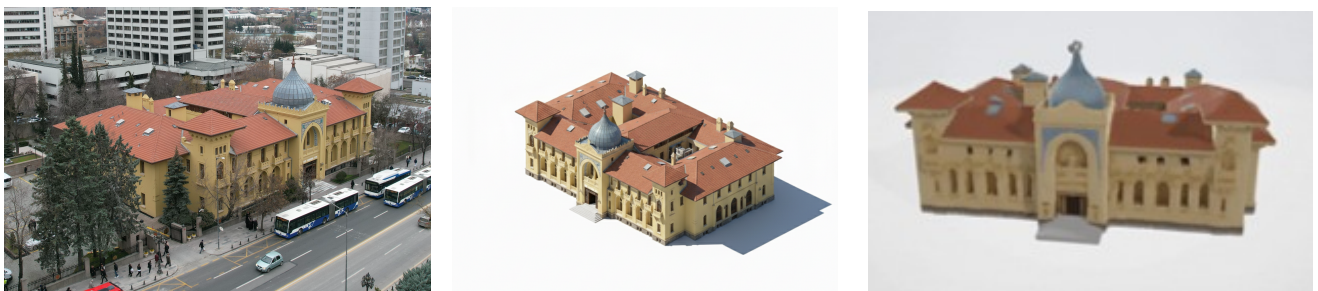
Figure 5. Three-step workflow of the proposed method illustrated using the Ankara Palace: (left) original building photograph, (centre) isometric daylight image generated by Gemini Flash 2.5, (right) textured 3D building model reconstructed by Hunyuan3D 2.1.
