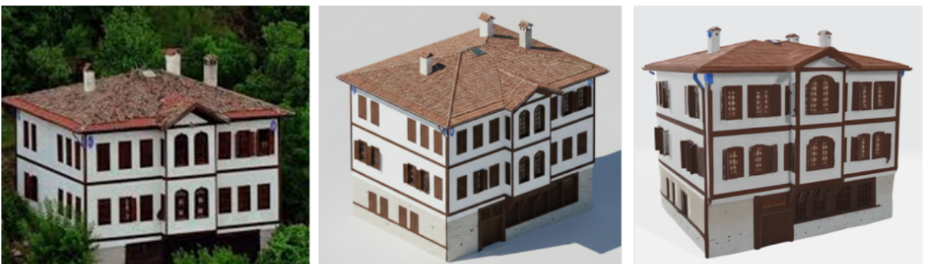
Figure 6. Three-step workflow of the proposed method illustrated using the Safranbolu House: (left) original building photograph, (centre) isometric daylight image generated by Gemini Flash 2.5, (right) textured 3D building model reconstructed by Hunyuan3D 2.1.
